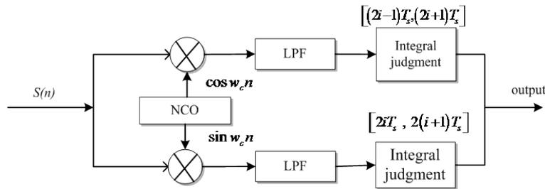
Fig. 1. The traditional demodulation method of MSK
