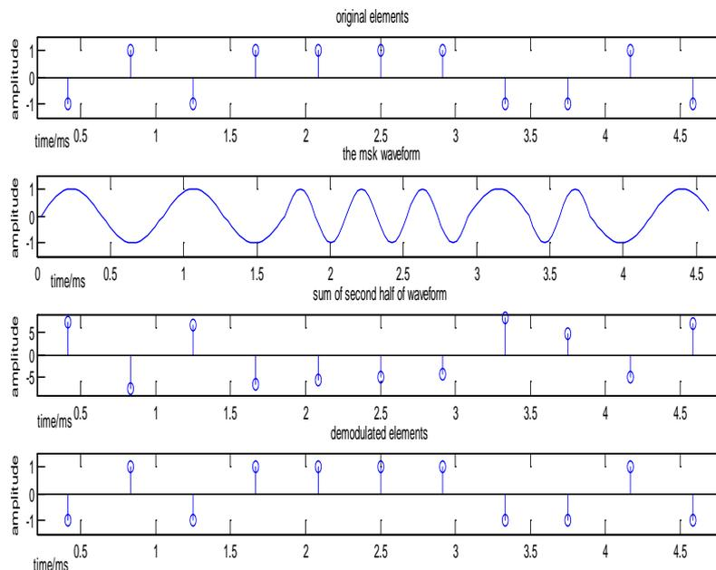
Fig. 3. The simulation of this demodulation method
