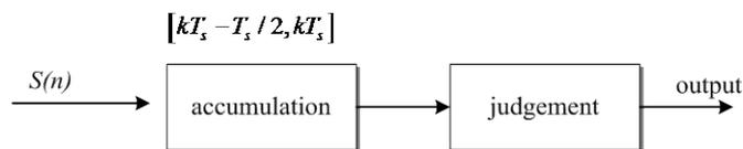
Fig. 2. The process of new demodulation method
