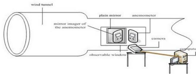
**Fig. 1.** Hardware structure of the system
