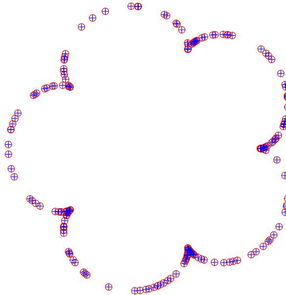
**Fig. 1.** Applying the tabu search algorithm to a 2D Bézier curve parameterization: original (red emptied circles) and reconstructed (blue + symbols) data points for the epicycloid curve.
