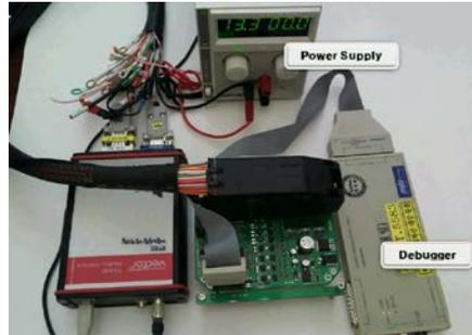
Fig. 5. Test bed for ECU Calibration.
