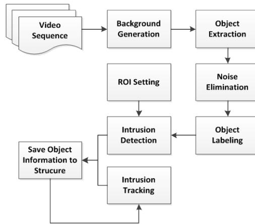
Fig. 1. The block diagram of Intrusion detection and tracking
