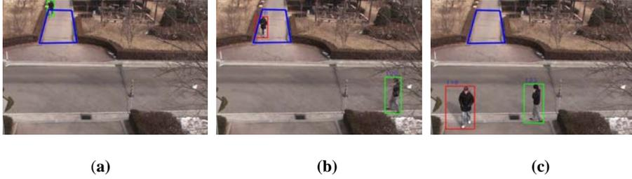
**Fig. 2.** The result of intrusion detection and tracking: ROI (blue box), intruder (red box), non-intruder (green box)
