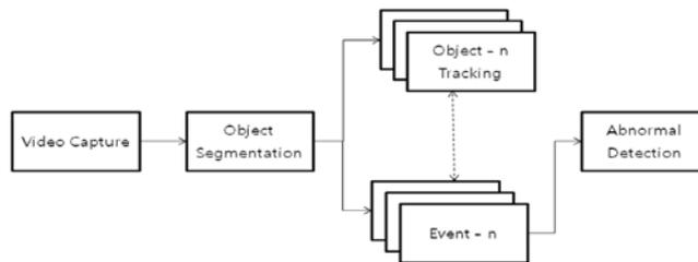
**Fig. 1.** The block diagram of An abnormal behavior detection based on image processing
