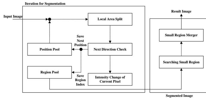
Fig. 1. Block diagram of the proposed region segmentation
