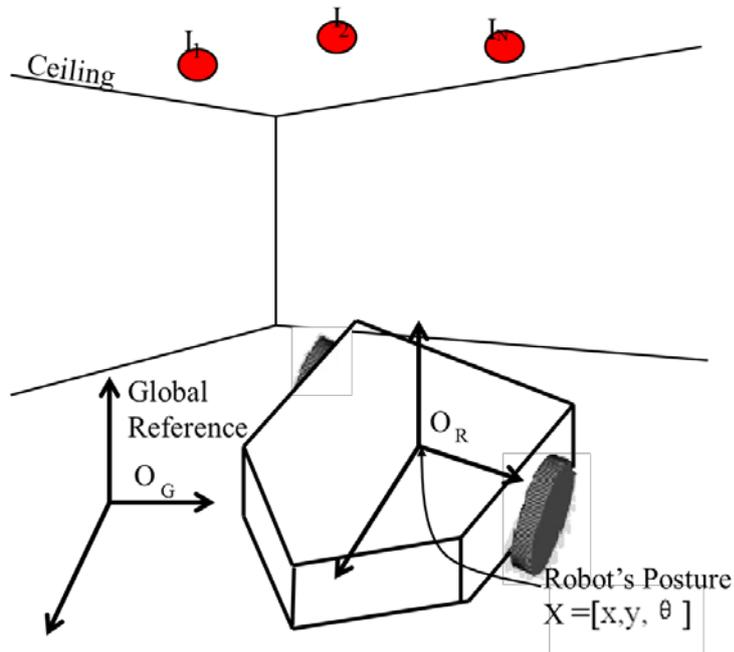
**Fig.1.** Vision based self-localization. The global coordinate origin  $O_G$ , the robot's current posture  $X$ , the interest point  $I_i$ . The arrows of the interest points represent their global direction.
