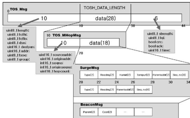
**Fig. 1.** The message structure of Tiny-OS
