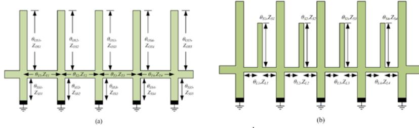
**Fig. 2.** Structure of (a) the  $\lambda_g/4$  short-stub BPF with 5<sup>th</sup> order and (b) the proposed harmonic suppressed BPF with the T-type inverter
