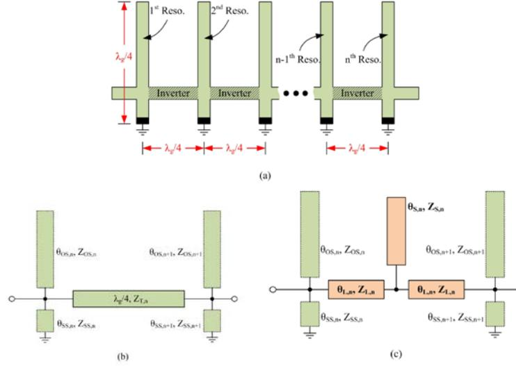
**Fig. 1.** Schematic of (a) the conventional narrow-band short-stub BPF using tapped-line geometry, (b) the quarter wavelength transmission line as the  $n$ 'th inverter, and (c) the T-type inverter as alternating by the T-type equivalent circuit for the quarter wavelength transmission-line
