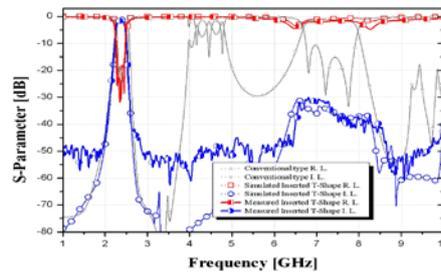
Fig. 4. Simulated and measured results of frequency responses for the harmonic suppressed short-stub BPF with T-type inverter
