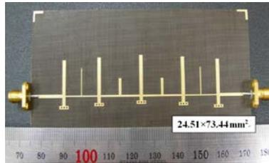
Fig. 3. Fabricated harmonic suppressed short-stub BPF with T-type inverter
