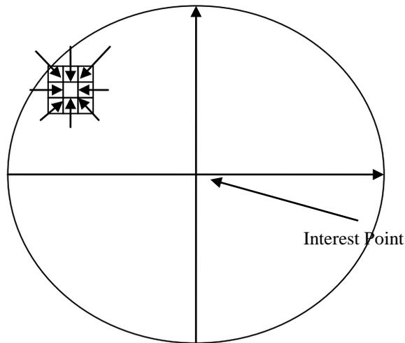
**Fig. 1.** Calculation of Descriptor. The descriptor is created by calculating the influence at each interest point of image in a neighborhood around interest points.
