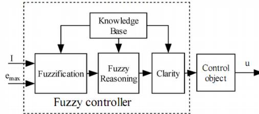
**Fig. 1.** The complicated equilibrium control problem of the battery pack can be simplified to a dual-input and single-output control. This paper has introduced the energy closed-loop control model based on fuzzy control strategy controller.
