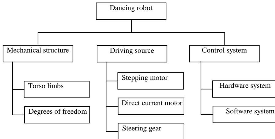
Fig. 1 The framework of system design
