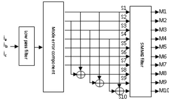
Fig. 1. Block diagram of the phase selection.
