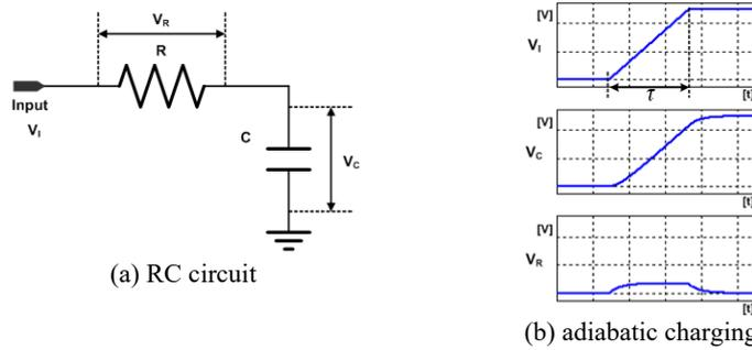
Fig. 1. Operation of the RC circuit
