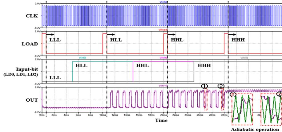
Fig. 3. Waveform of 3-bit digital PWM using ADCL without  $C_S$
