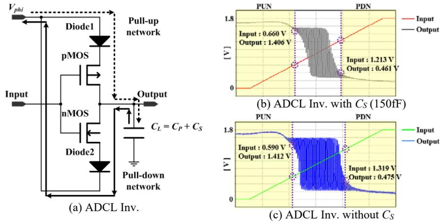
Fig. 2. ADCL Inverter
