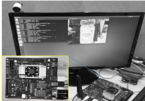
Fig. 2. Classification Test for the compressed GoogleNet on embedded system
