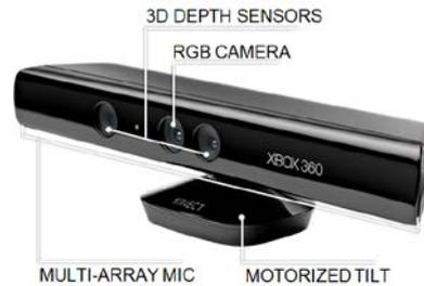
**Fig. 2.** Microsoft Kinect Sensor
