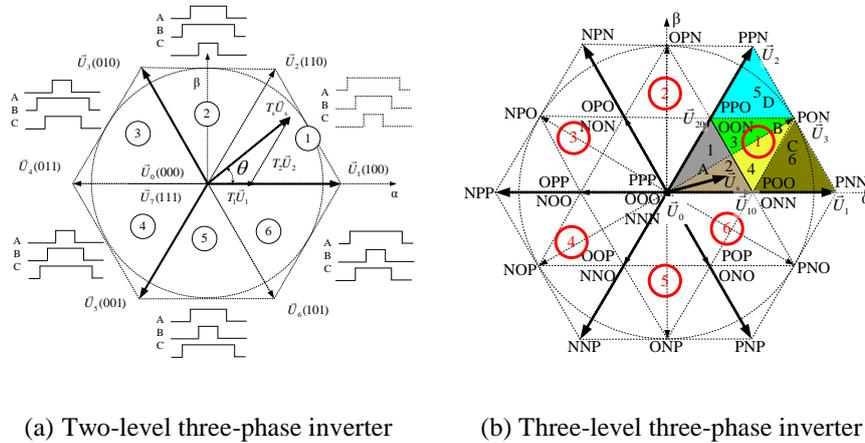
(a) Two-level three-phase inverter (b) Three-level three-phase inverter
