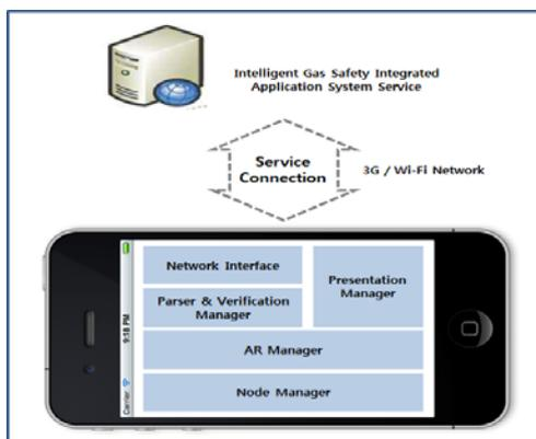
**Fig. 1.** Mobile system architecture
