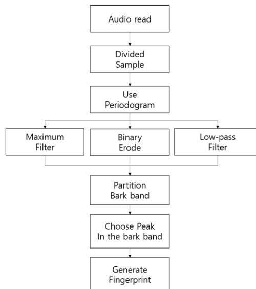
**Fig. 2. The process of the proposed method**
