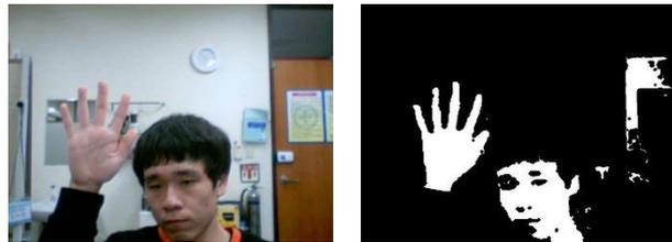
**Fig. 1.** This shows a result of skin color detection. We can segment skin color regions properly in indoor environment, as shown in the right image.
