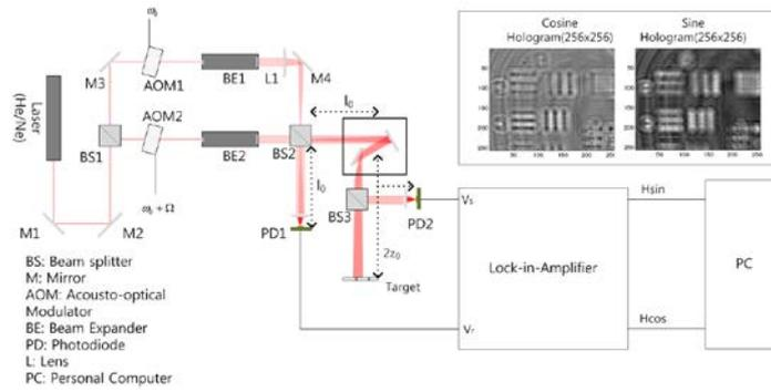
**Fig. 1.** Experimental setup (subset: the sine and cosine hologram)
