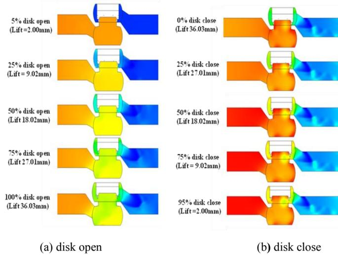
**Fig. 2.** Pressure distribution with disk open and close
