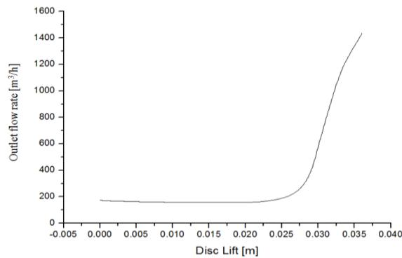
**Fig. 3.** Outlet flow rate with disk lift variation.
