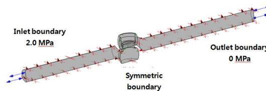
**Fig. 1.** Boundary conditions of model
