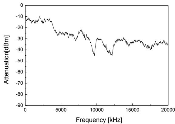
Fig. 3. Attenuation measurement schematic diagram at all bands at 10 m
