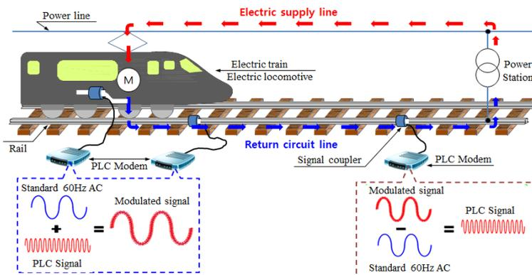
Fig. 1. The schematic diagram of concept on rail track PLC
