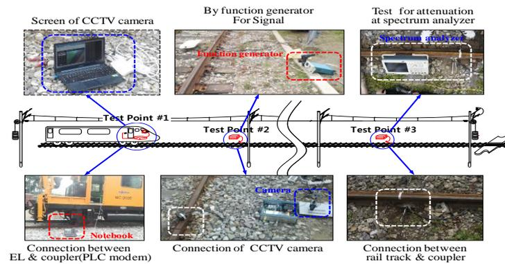
Fig. 2. Actual measurement experiment and schematic drawing of rail track PLC
