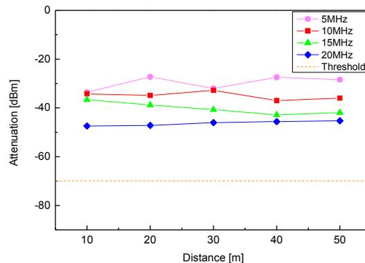
Fig. 4. Attenuation variation with track distance
