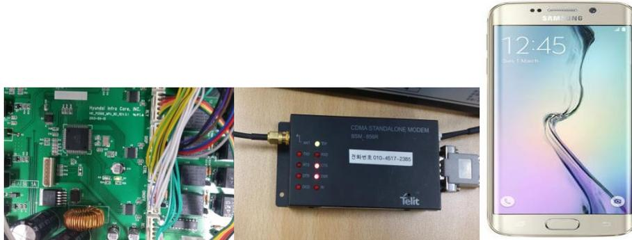
**Fig. 8.** System of the smart applications: (a) MPU board of the receiver (b) CDMA module (c) smart phone
