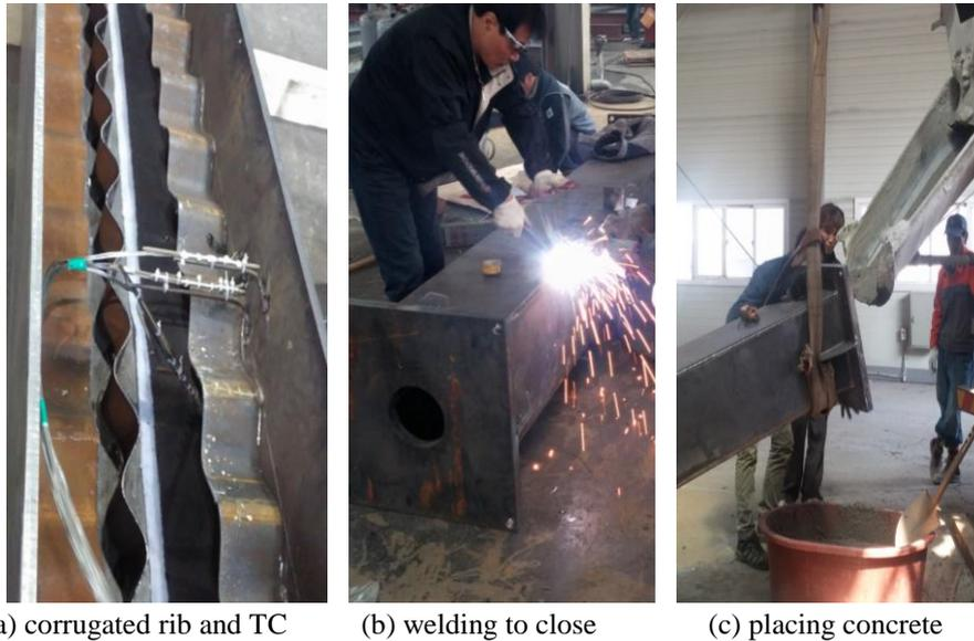
**Fig. 1.** Process to fabricate CFT specimen
