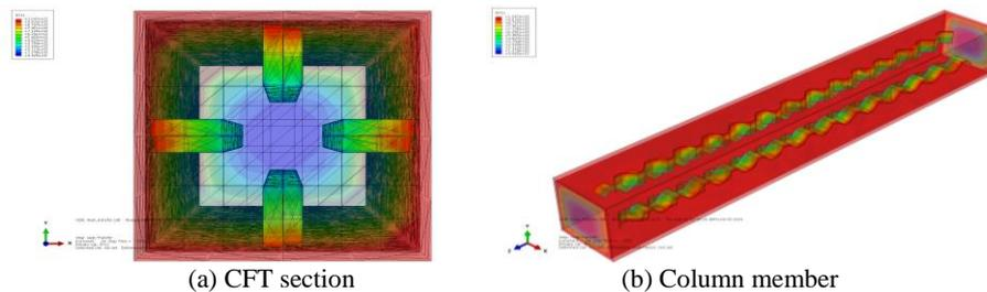
Fig. 4. Temperature distribution analysis on the CFT specimen
