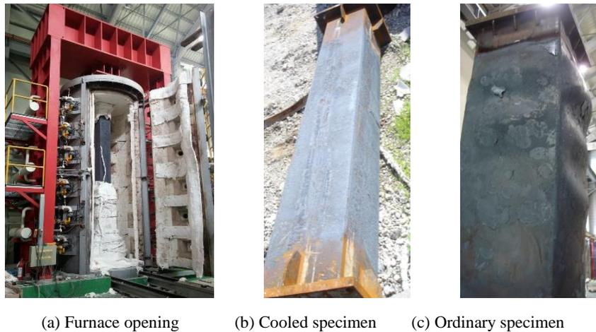
**Fig. 3.** Comparing the failure mode between this study and ordinary CFT columns
