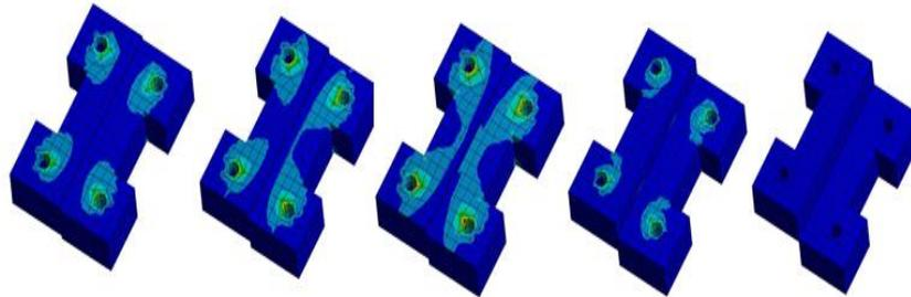
**Fig. 4.** Change of the equivalent stress according to the progress of forced displacement (*Thickness of specimen is 35mm*)
