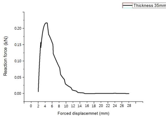
Fig. 3. Graph of reaction force due to forced displacement at static analysis(Thickness of specimen is 35mm)
