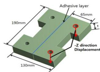
Fig. 1. Mode III-type specimen model
