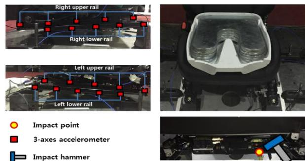
Fig. 2. Test set up for the modal test of seat slide rail.
