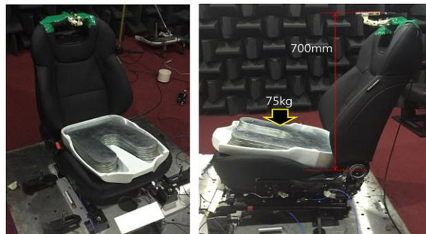
Fig. 1. Test set up for measurement of seat slide operating noise.
