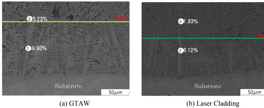
Fig. 2. Microstructure on coating layer
