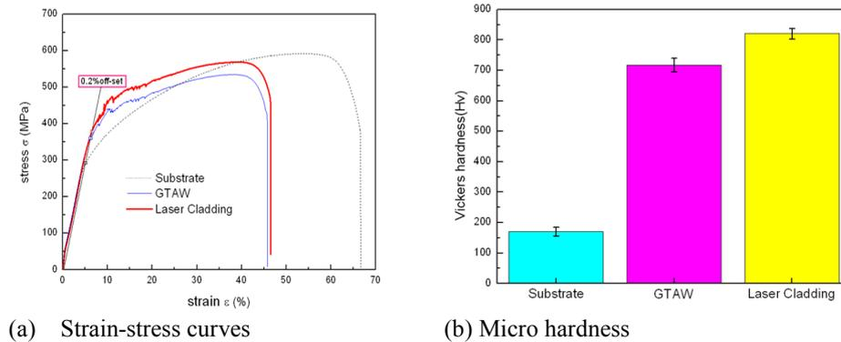
Fig. 1. Mechanical properties
