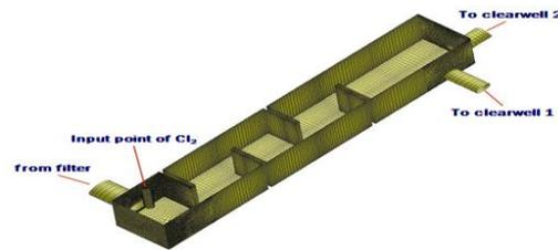
Fig. 2. Model of influx in clearwell
