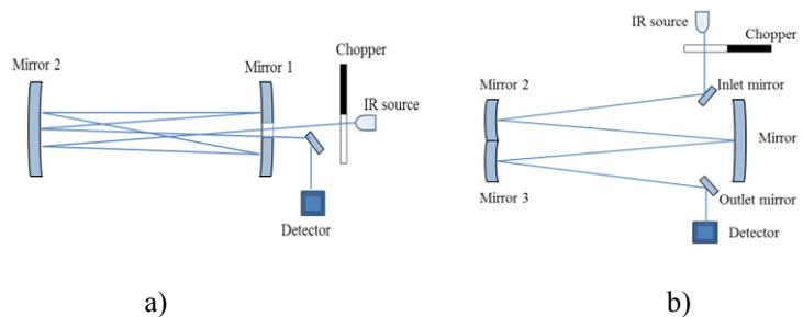
Fig. 2. Experimental set-up of Herriott cell (a) and White cell (b).
