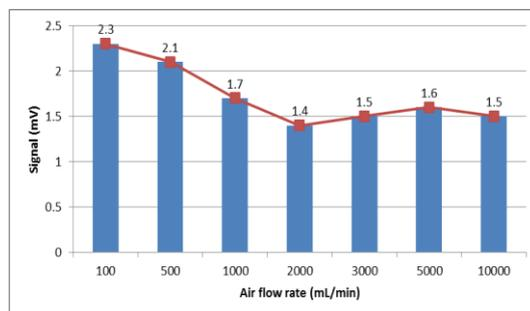
**Fig. 8.** The relationship between gas flow rate in the gas cell and detector signal.
