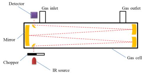
Fig. 1. A structure of an NDIR.
