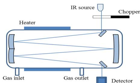
**Fig. 3.** Experimental set-up for gas cell temperature and optimal operation.
