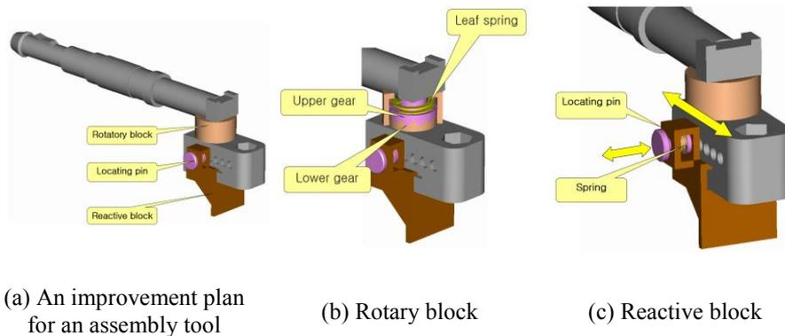
Fig. 1. Structure of Improved Assembly Tool
