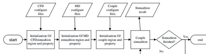
Fig. 1. Flowchart of Micro-Macro coupled solver
