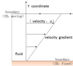
Fig. 2. Illustration of Couette flow field
