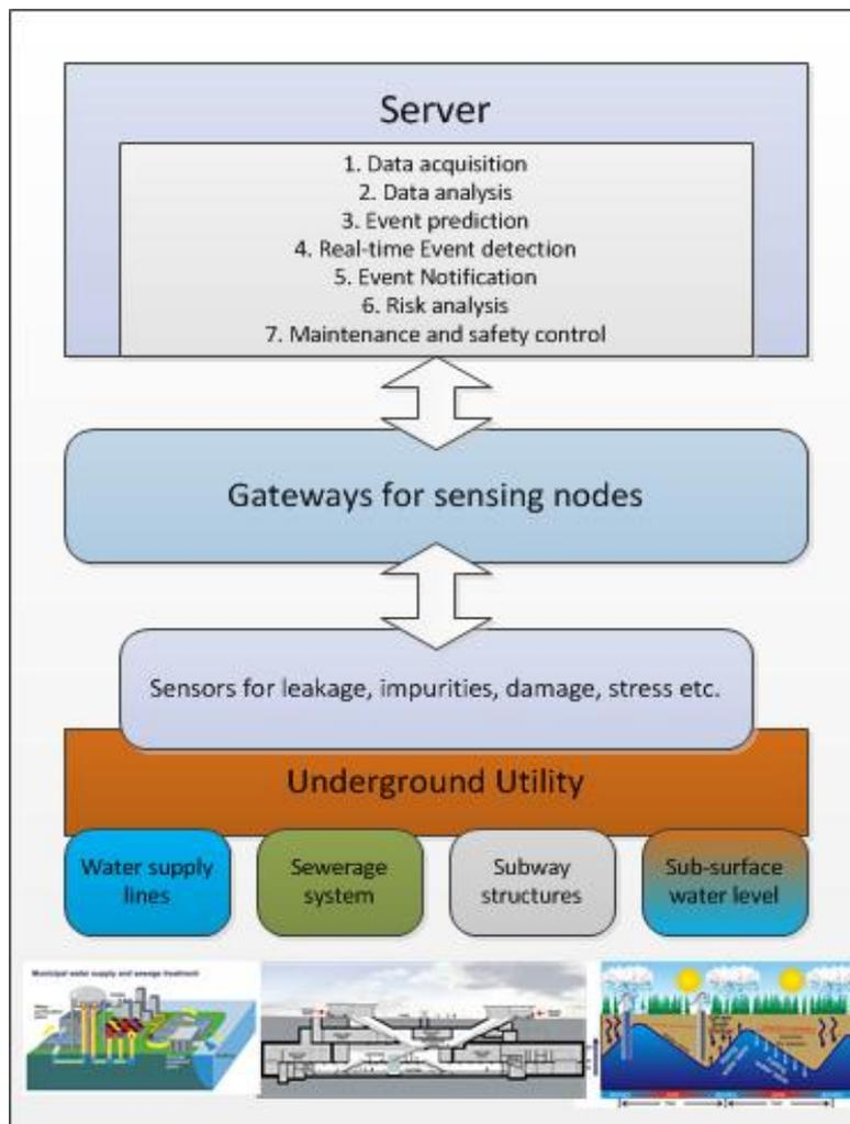
**Figure 1.** System architecture for the underground facility monitoring
