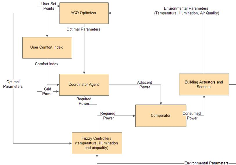
**Fig. 1.** Efficient optimization approach based on ACO algorithm for energy management in building environment
