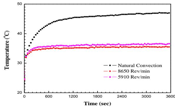
**Fig. 3** Junction temperature distribution for different fan speeds at constant input power of 5.75 W
