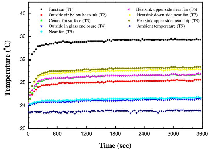
**Fig. 5** Temperature distribution at different locations with input power 5.75 W and fan speed 4030 rev/min
