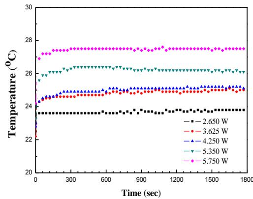
**Fig. 4** Junction temperature for different input power at constant fan speed of 5750 rev/min
