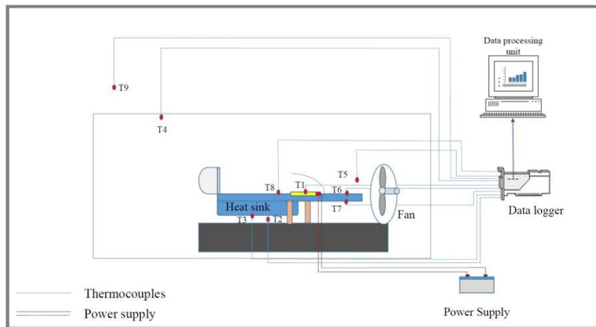
**Fig. 1** Schematic of experimental setup with thermocouple locations
