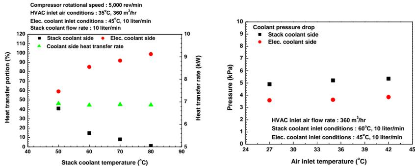
(a) Heat transfer rate portion among triple fluids (b) Pressure drop for coolants
