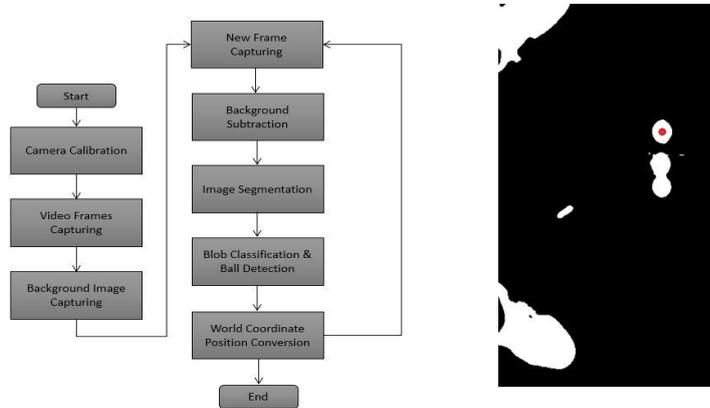
**Fig. 1.** Golf ball detection algorithm and detection result
