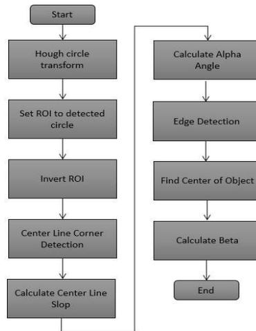
**Fig. 4.** Algorithm of ball roll and pitch calculation
