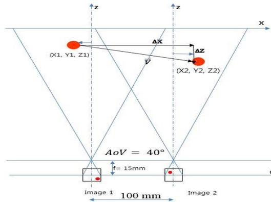
Fig. 6. Stereo vision schematic
