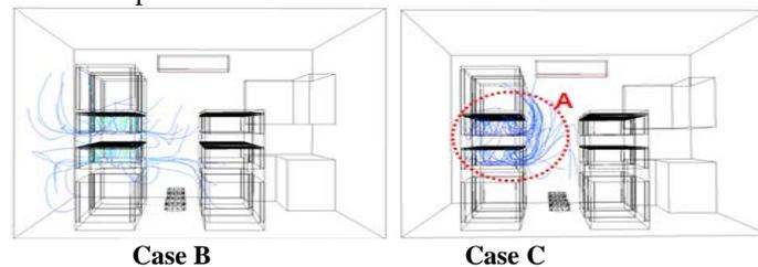
Fig. 2. Air flow distribution according to control conditions
