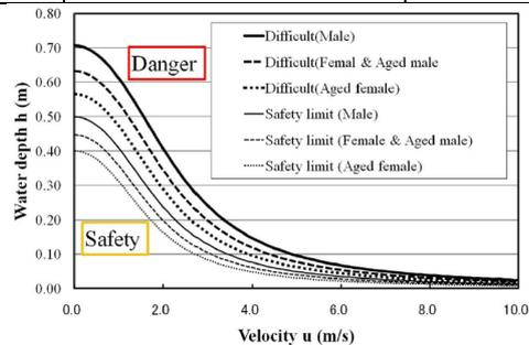
**Fig. 1.** Criteria of safe evacuation described by water depth and velocity [3]
