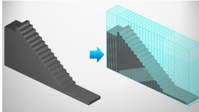
**Fig. 2.** Geometry and mesh generation of the stair model
