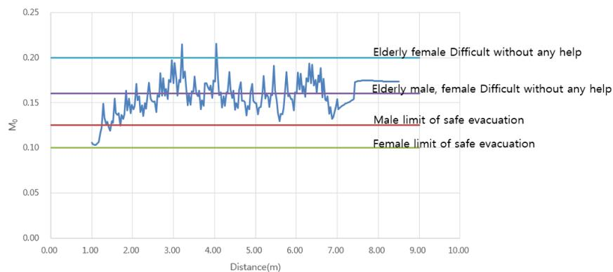
**Fig. 3.** 3D Specific force evaluation ( $Q=0.5 \text{ m}^3/\text{s}$ )
