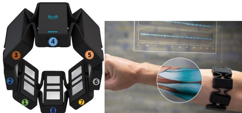
Fig. 3. Myo armband and the number of sensors.
