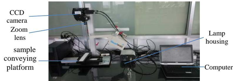
**Fig.1.** Hyperspectral image system
