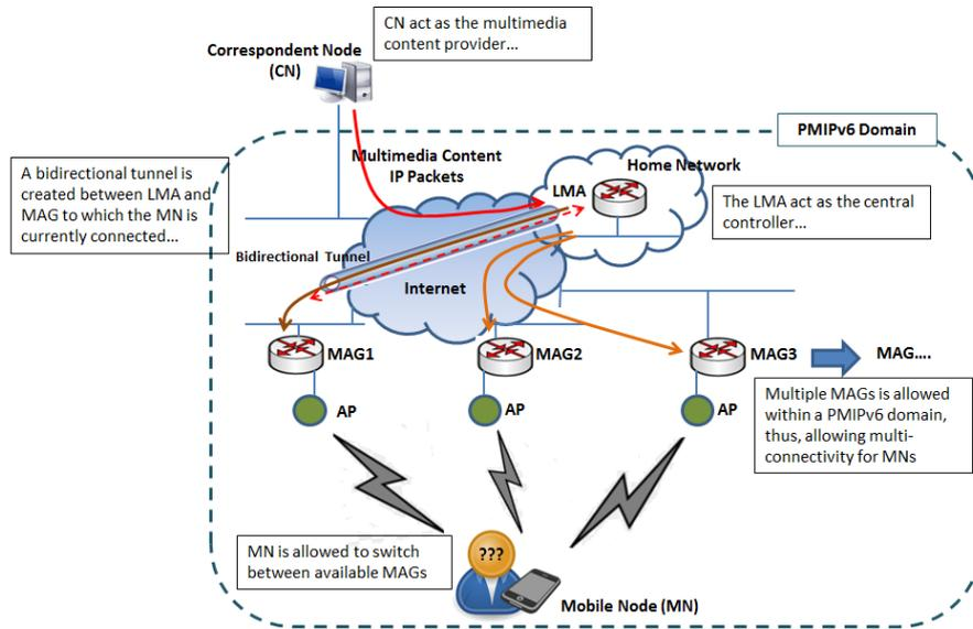
**Fig. 1.** Mobile Node Chooses Connection Considering the Handover Latency based on the Current Traffic among Heterogeneous Networks
