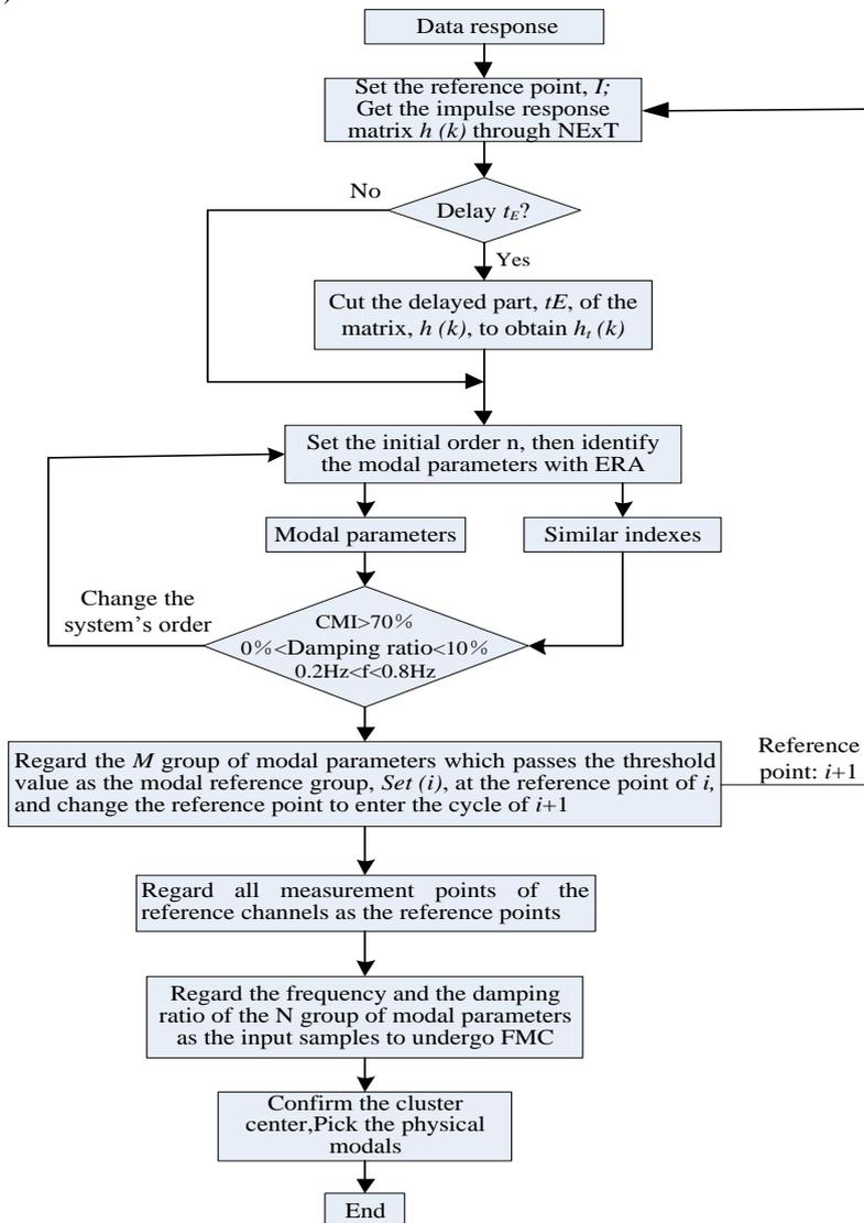
Fig. 1. The flowchart of automatic identification algorithm
