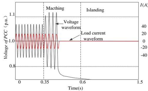
**Fig.3:** Waveform of active current disturbance
