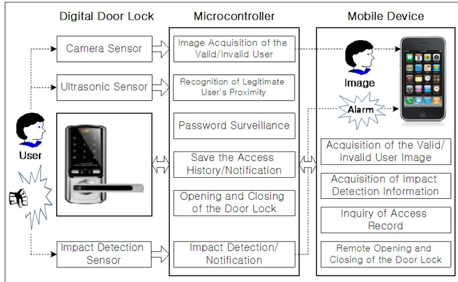
**Fig. 1.** Structure of the proposed door lock system
