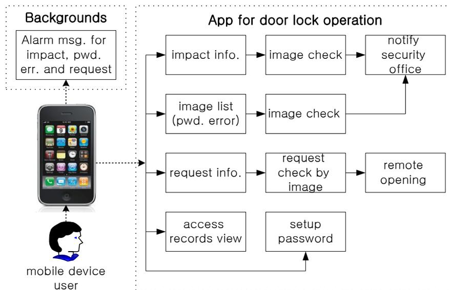
Fig. 2. Mobile app menu structure for digital door lock operation
