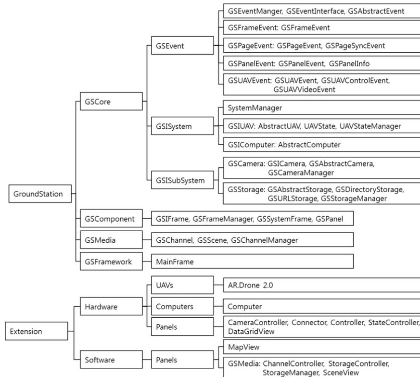
Fig. 3. Structure of the proposed ground station
