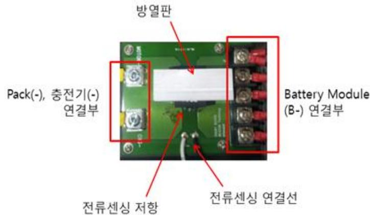
Fig. 3. Current Measurement System
