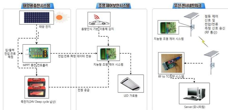
Fig. 1. Standalone Smart Solar-powered Streetlamp Light control System
