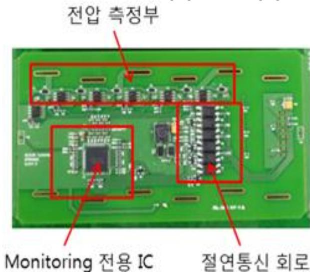
Fig. 2. Voltage Measurement System
