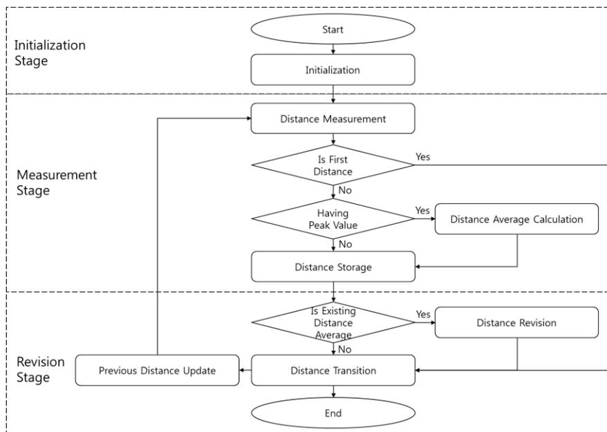
Fig. 1. The process of real-time distance revision
